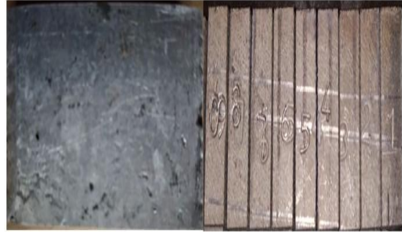
Fig.1. Inconel alloy before and after machining
