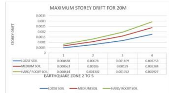
Graph No. 4 MAXIMUM STOREY DRIFT FOR 20M
