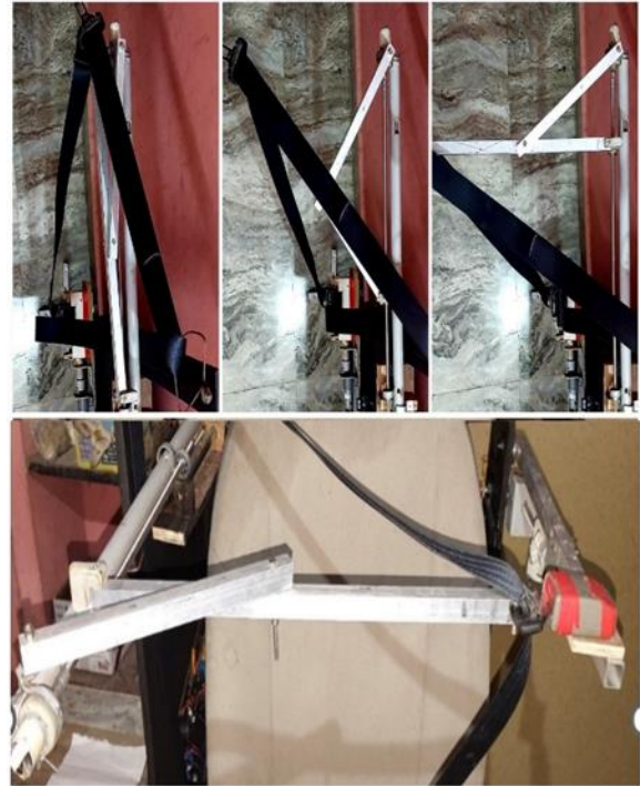
Fig 4.2: Working of Single scissor mechanism
