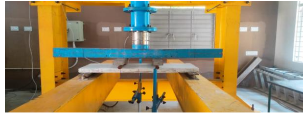
Fig. 3 Experimental Setup For Flexural Test On Ferrocement Slab
