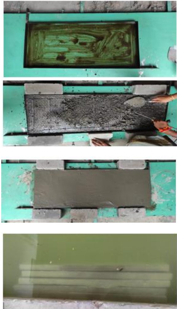
Fig. 2 Preparation Of Mould Casting & Curing Of Slab
