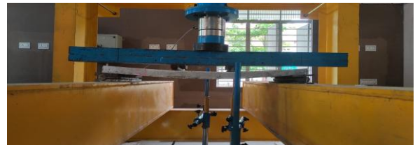
Fig. 4 Flexural behaviour of Ferrocement Slab
