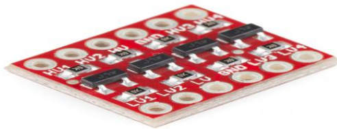
Figure 4: Logic converter (5 to 3.3V)
