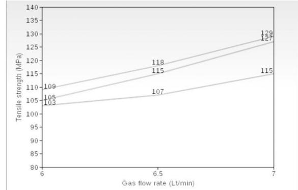
Figure 4.1 Ultimate Tensile Strength variation as a Function of Gas Flow Rate
