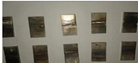
Figure 4.5 Hardness Test Specimens
