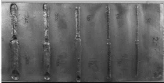
Figure 3.3 (a) TIG welded stainless steel types
