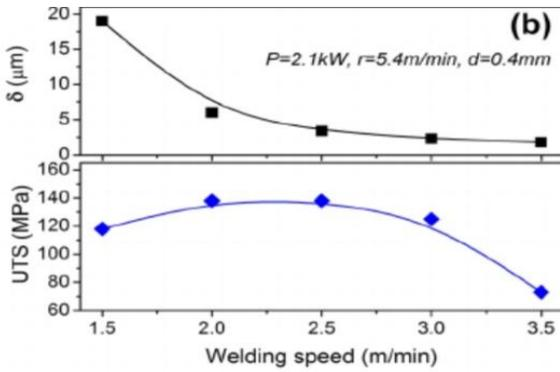
Figure 4.2 Variation in specimen ultimate tensile strength as a function of welding speed
