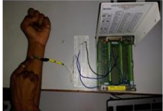
Fig 10. Acquisition of Pulse Signal
