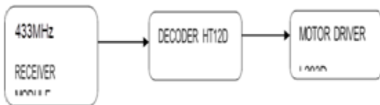
Fig 1.0 Block Diagram of the wireless gesture controlled robot
