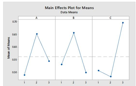
Fig. 5. Main Effect Plot for Cu nanofluid + MQL Machining Environment
