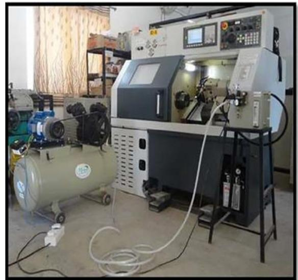
Fig.1. Experimentation Setup with MQL System
