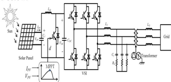
Fig.1 Block diagram of 3 phase grid integrated PV system
