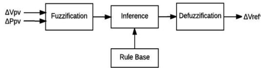
Fig. 6 Fuzzy logic control diagram
