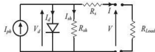
Fig. 2 Typical circuit of Solar PV cell
