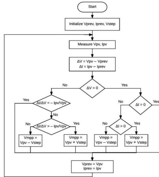
Fig. 5 Flow chart of incremental conductance method.
