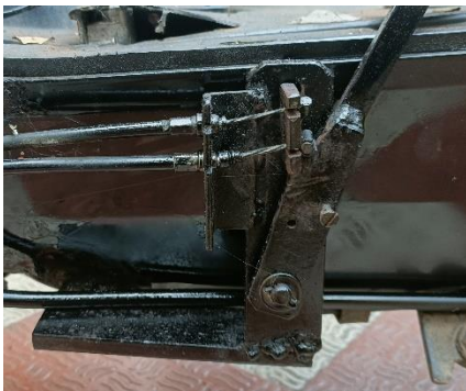
Fig 4: Brake pedal mechanism (E-shaped plate)
