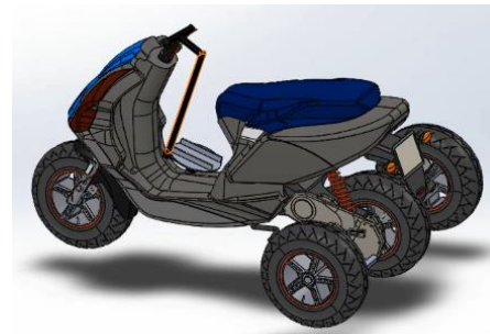
Fig.2: CAD model of Scooter and Steering mechanism
