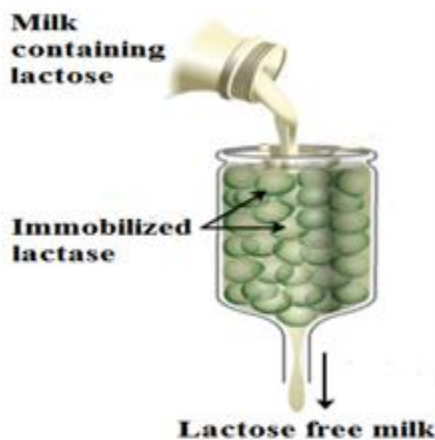
Figure 7: The immobilized enzyme converts lactose into glucose and galactose as the milk flows through.
