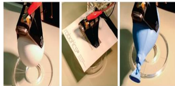
Fig 7. Dielectric gripper lifting various sized objects [5]
