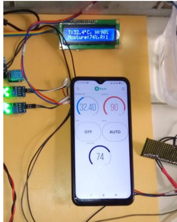
Fig. 8: The output of the project when the water pump is switched on automatically.
