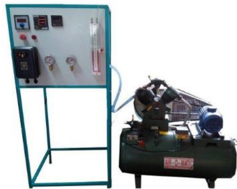
Fig. 1. Experimental set-up of reciprocating air compressor
