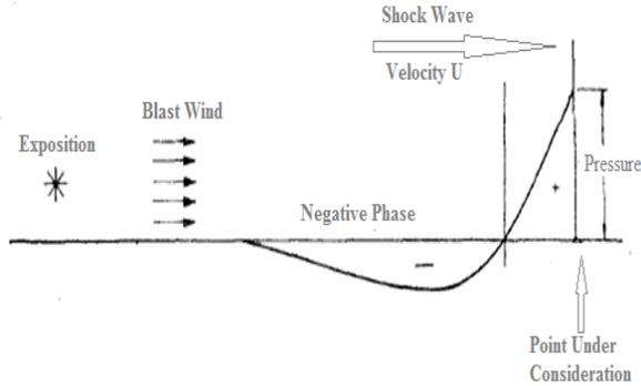
Figure. Shock Wave produced by Blast
