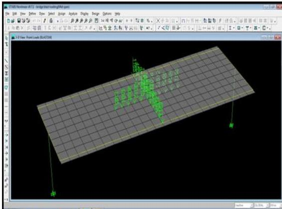
Figure. Blast Load Distribution for Case 1 in ETABS
