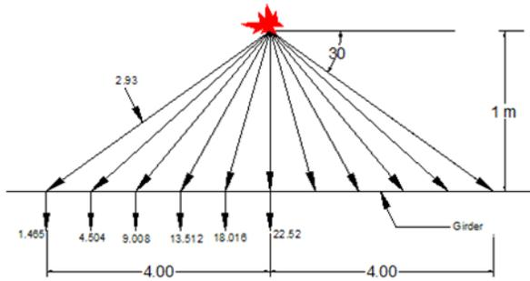
Figure. Blast pressure distribution for Case 1
