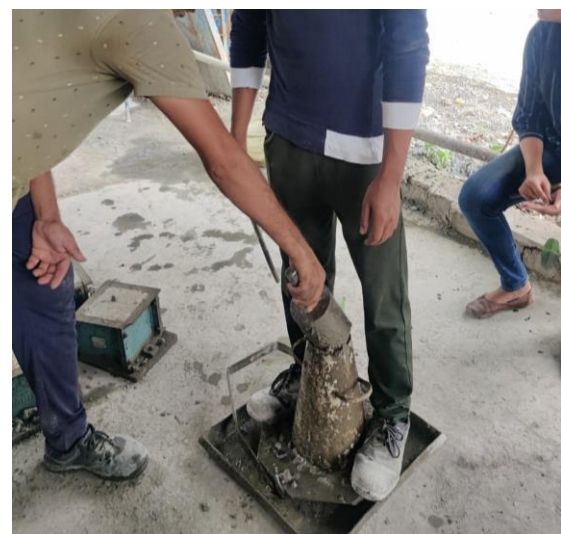
Figure 3: Slump Cone Test
