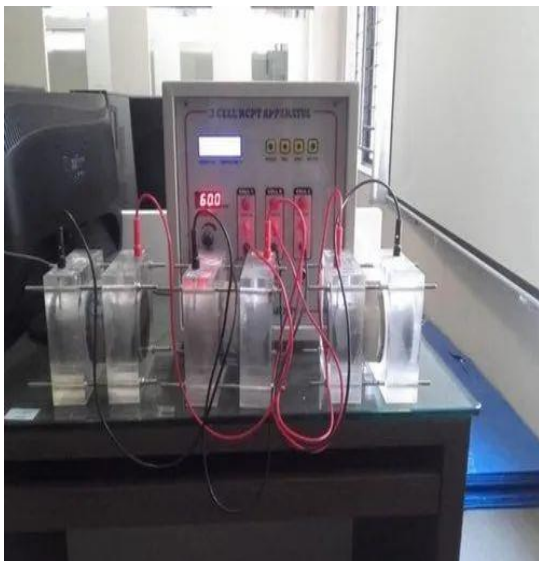
Figure14: RCPT testing of concrete
