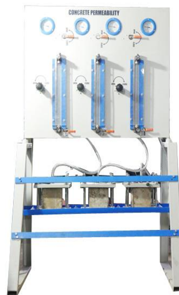
Figure 17: Water Permeability test
