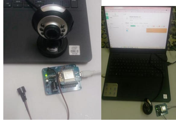
Fig 11 Hardware Setup for IoT integration using Node MCU and PC
