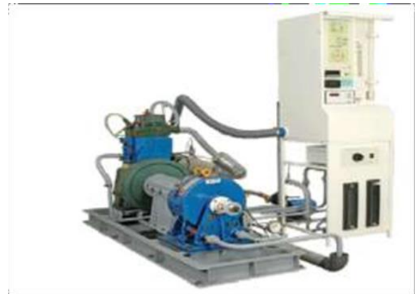
Fig-4: Computerized Single cylinder 4 stroke Diesel engine(VCR engine)
