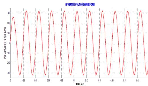
Figure 12. Waveform of a Single Phase Voltage Source Inverter
