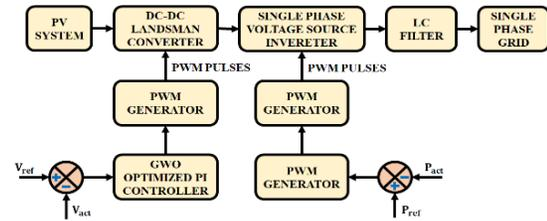
Figure 1. Proposed System Block Diagram
