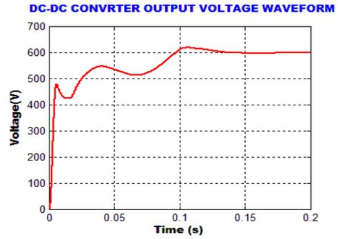
Figure 10. DC-DC Converter Output Voltage Waveform
