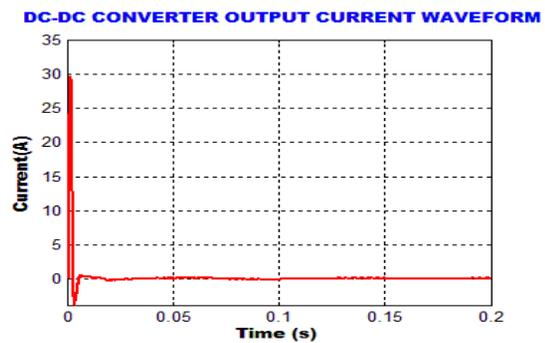
Figure 11. Dc-Dc Converter Output Current Waveform
