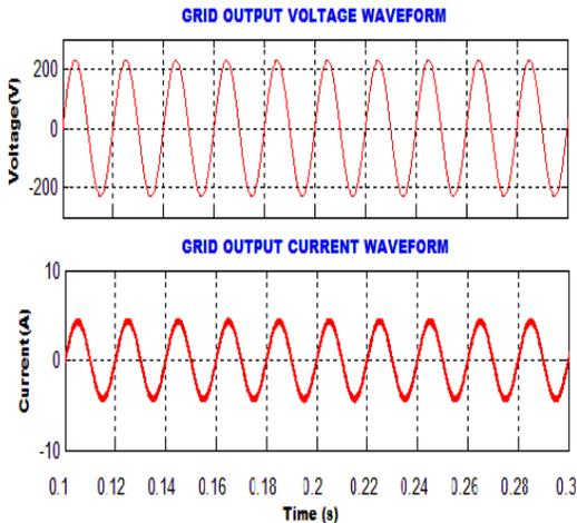
Figure 13. Single Phase Grid Output Waveform
