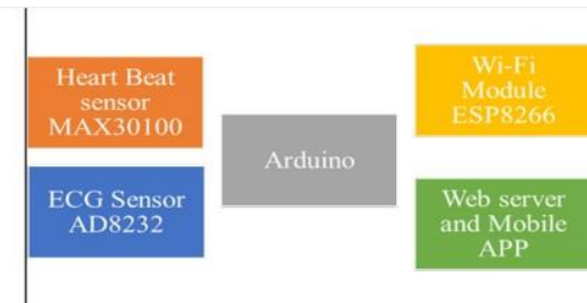
Fig. 2 shows the design of the IoT device-based ECG system
