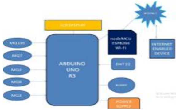
Fig. 3: Block diagram of proposed model
