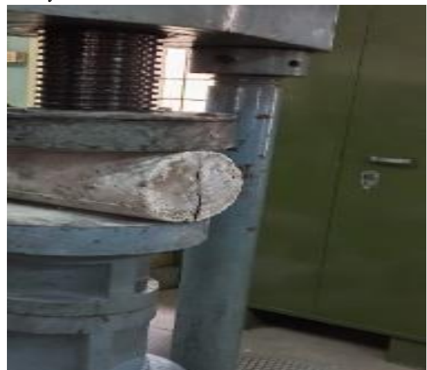
FIG 2 SPLIT TENSLE STRENGTH OF SCC
