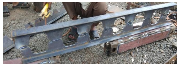
Figure No.4 Grinding of castellated beam IV) Colouring – It's last part of castellation of the entire beam because it is good finishing and attractive surface of this beam. It is also helping the easily naming on the beams with help of marker.
