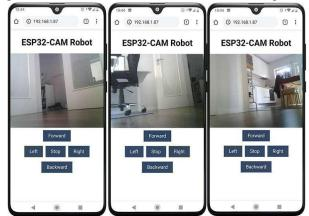
The surveillance bot ESP32-CAM module has an ESP32-S processor, an OV2640 camera, and a microSD card slot. Images captured by the camera can be stored on a MicroSD card slot. The HTTP communication protocol will be utilized to receive video streaming from the OV2640 camera via a web browser in this case. As indicated in the image above, the webpage will also feature buttons to move the car in the Left, Right, Forward, and Reverse directions.
