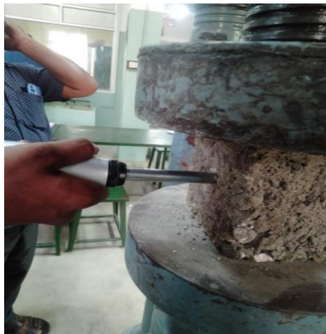
fig 8.1 rebound hammer test
