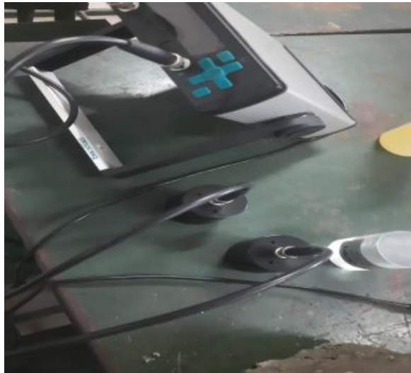
Fig no 8.2 ultrasonic pulse velocity test
