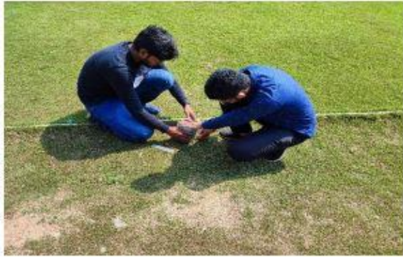
Figure 9: Digging the soil for setting up Infiltrometer The rate of water infiltration into soil in a limited area is measured using a single-ring infiltrometer. It consists of a single metal ring that is driven into the soil's surface to form a circle, usually having a diameter of 30 to 60 cm. The base of the ring is flat and smooth, which makes it easier for water to be distributed evenly throughout the soil.
