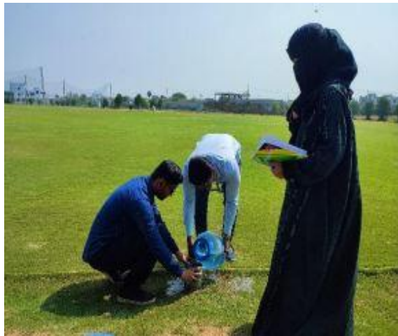
Figure 10: Filling the water in Infiltrometer Table 2: Infiltration Test Results
