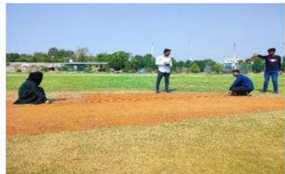
Figure 7: Ranging and measuring the diameter of the stadium using Tape
