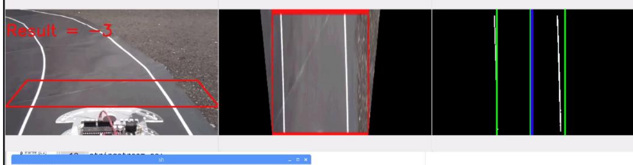
Figure2: - It indicates that the vehicle moved right because of -3 or negative result.
