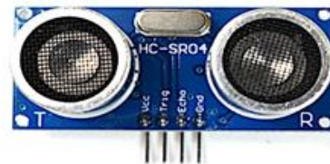
Fig 4: Ultrasonic distance sensor
