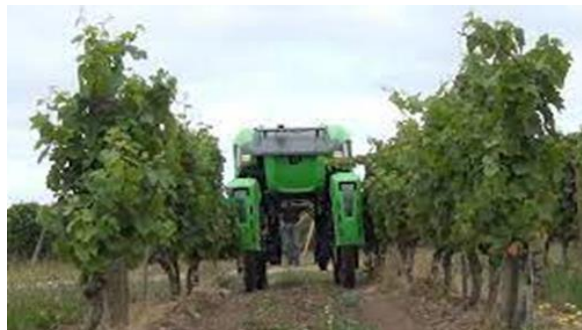
Fig. 5 Sitia Trektor Fertilizer Spraying Robot Resizing of the machine is possible in different dimensions, therefore is likely to be able to fit a field customized.
