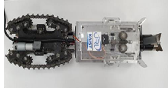
Fig. 4 (a) Mole-bot (Digging Robot), (b) Mole-bot. Mole-bot (Fig. 4a) includes a stout scapula, a waist which inclines all sides, and forelimbs that are powerful. However, the most significant feature of it is the powerful torque from the expandable drilling bit which mimics the chiselling ability of that of a mole's front teeth, which highlights as the best feature of this drilling robot.
