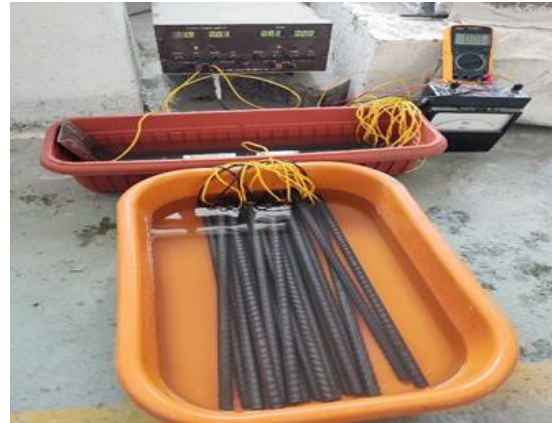
Fig 6 Accelerated corrosion setup
