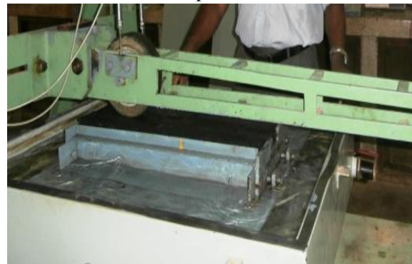
Fig.1. Testing of Specimen in Immersion Wheel Tracking Device
