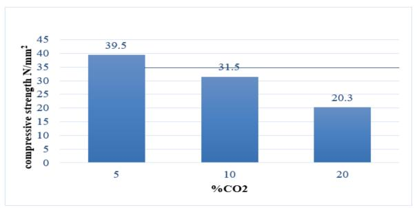
Compressive strength of 5%, 10%, 20% of CO<sub>2</sub> in concrete decrease gradually. For 5% of CO<sub>2</sub> in concrete increase the compressive strength compared to conventional concrete.
