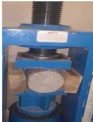
Figure 4 Tensile testing of specimen
