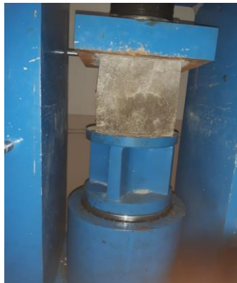
Figure 3 Compressive testing of specimen testing on beam
