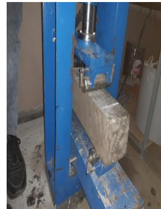
Figure 5 Flexure testing on beam
