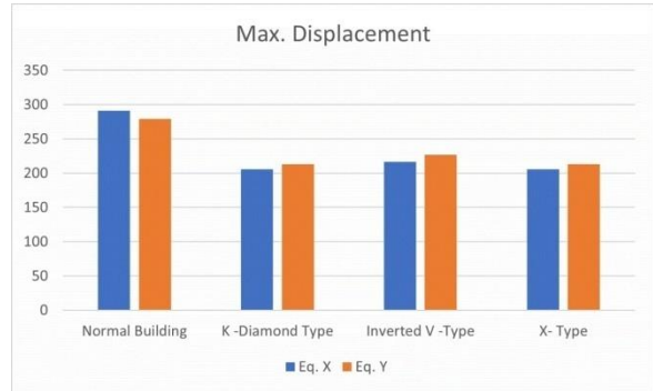
Fig.3 (b) Story Displacement for bracing system
