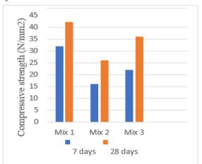
This graph shows that the compressive strength of Mix 2 is very low. Compared to Mix 2, Mix 3 have high compressive strength value. It achieves by the addition of jaggery.
