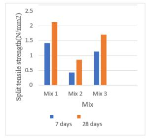
This graph shows split tensile strength of Mix 3 is relatively higher than Mix 2. By adding jaggery, strength value can be increased up to a certain limit.
