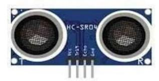
Principle: Ultrasonic sensors consist of a transmitter and a receiver. The transmitter emits ultrasonic Operating waves, usually in the frequency range of 20 kHz to 200 kHz, and the receiver detects the waves after they bounce off objects in their path.
