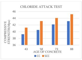
The tested values of B-Acid attack test, C-Sulphate attack test, D-Chloride attack test are listed below
