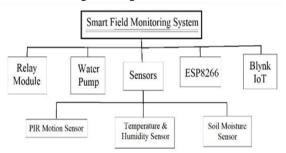
The NodeMCU microcontroller was programmed using an appropriate programming language (e.g., Arduino IDE). The programming code included instructions to read sensor data at regular intervals, process the data, and transmit it to the Blynk IoT platform via a stable internet connection. The code also incorporated functionalities to handle motion detection events and trigger alerts when necessary.
