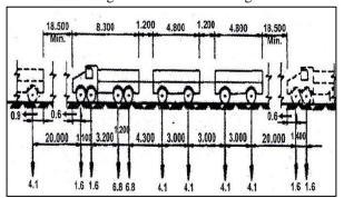
Fig 4 IRC Class B loading
