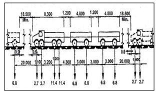
Fig 3 IRC Class A loading
