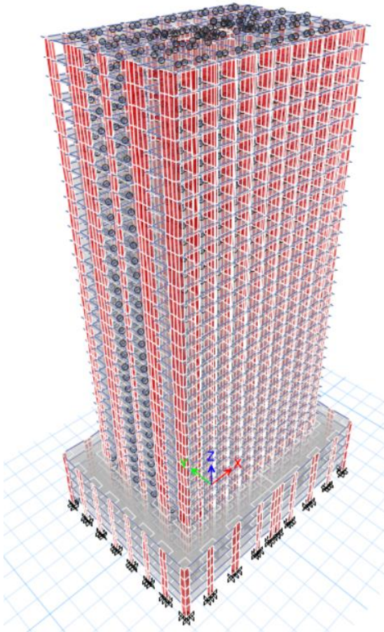
Figure 4.2 Tower + Non tower ETABS 3D model
