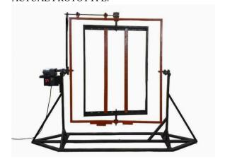
The fact that the mould rotates at a comparatively sluggish pace—typically up to 12 rev/min— should be noted. Therefore, the procedure should not be confused with centrifugal casting, in which the plastic is flung against the mould wall as the mould rotates rapidly. While it may seem appealing to spin the mould quickly in order to boost output, the intricate
