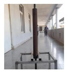
The hub in a vertical axis wind mill serves as a critical interface between the rotor blades and the main shaft of the turbine. It provides structural support, facilitates rotational motion, and ensures efficient energy conversion from wind to mechanical power. Proper design and construction of the hub are essential for optimizing the performance, reliability, and longevity of the VAWT system.
