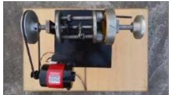
Fig 6 Fabricated Eclipse Gear Box Model With Two Linkages
