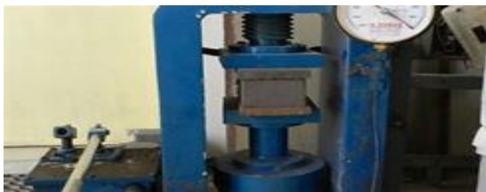
Figure(d): Cubes tested under compressive testing
