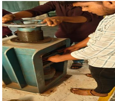
Figure(e): Cubes tested under compressive testing machine.
