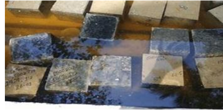
Figure(d): Curing the cubes for 7, 14, & 28 days.
