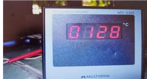
Fig-4: Photographic view of digital temperature indicator
