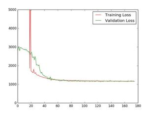
4. This graph illustrates a situation in which there are no overfitting or underfitting problems during training, as the training loss and validation loss converge to comparable low levels.
