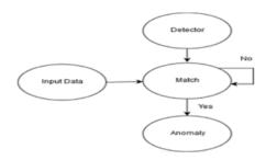
A botnet detection system's data flow diagram (DFD) is depicted in the picture. There are three primary processes involved: Data is first fed into the system during the input stage so that it can be analyzed.
