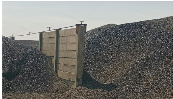
Photo 8, Water sprinkler installed in the batching plant raw material bins
