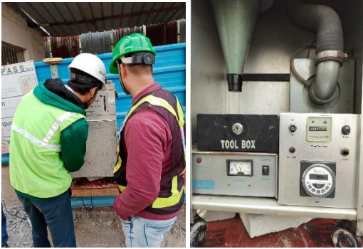
Photo 2, Ambient air pollutant sampler
