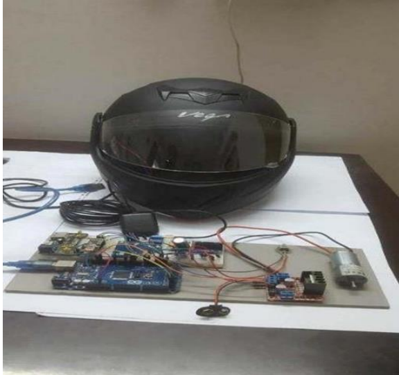
Fig. 1. Helmet with Receiver circuit
